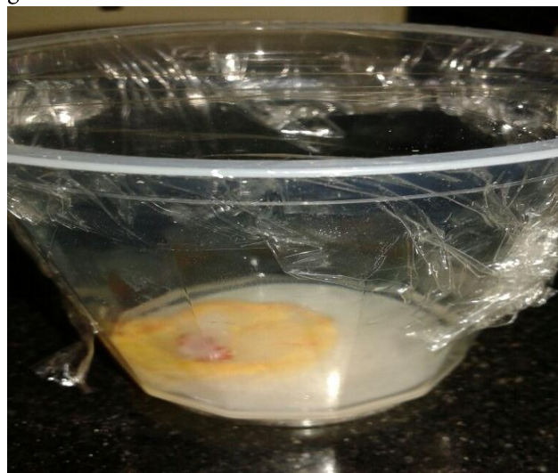
Figure 8: The assembly shows three distinct layer- Lowermost sponge layer Whatmann Filter paper in the middle Soft Agar layer on the top
